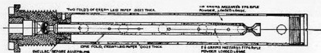
FIG. 2.—CASE PERCUSSION IGNITION PRIMER.
