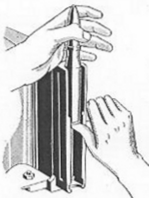
Figure 62—Unloading a fully tensioned magazine
