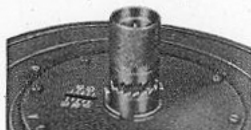
Figure 56. Coupling Sleeve Raised and Turned to Lock It Out of Engagement with Spring Axis.
