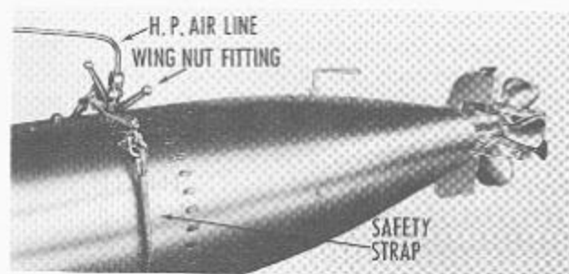
FIGURE 12C3.—Charging the air flask.
