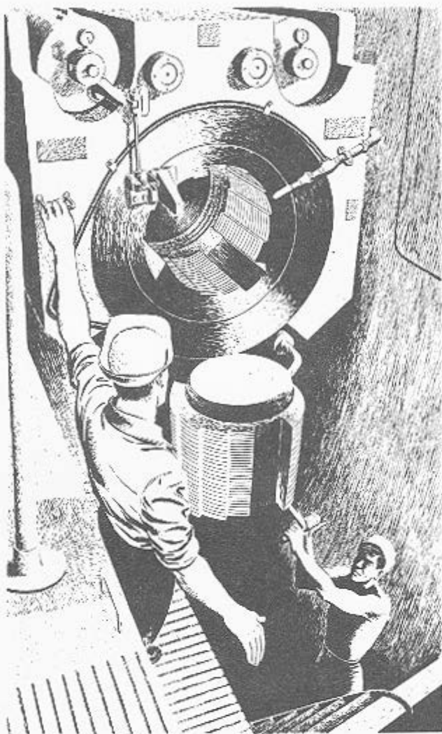
FIGURE 5B12.—Interrupted-screw type breech mechanism (16-inch) now used in the Fleet.
