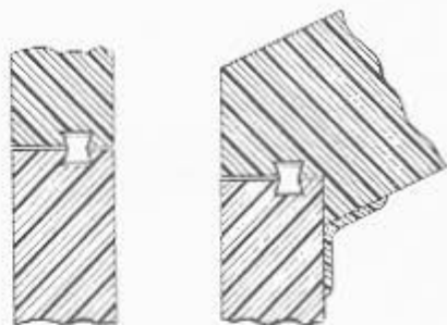
FIGURE 4A2.—Method of keying adjacent plates of Class A armor. Butt joint is shown at left—angle joint at right.
