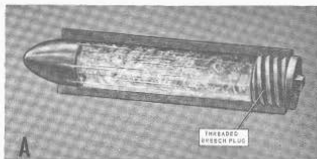
FIGURE 5B10.—Principle of the interrupted-screw breech-mechanism. A. Continuously threaded breech plug.
