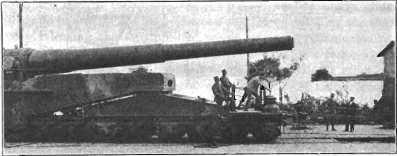
TRANSLATING MOUNT WITH HAND WINCH AND CABLE.
