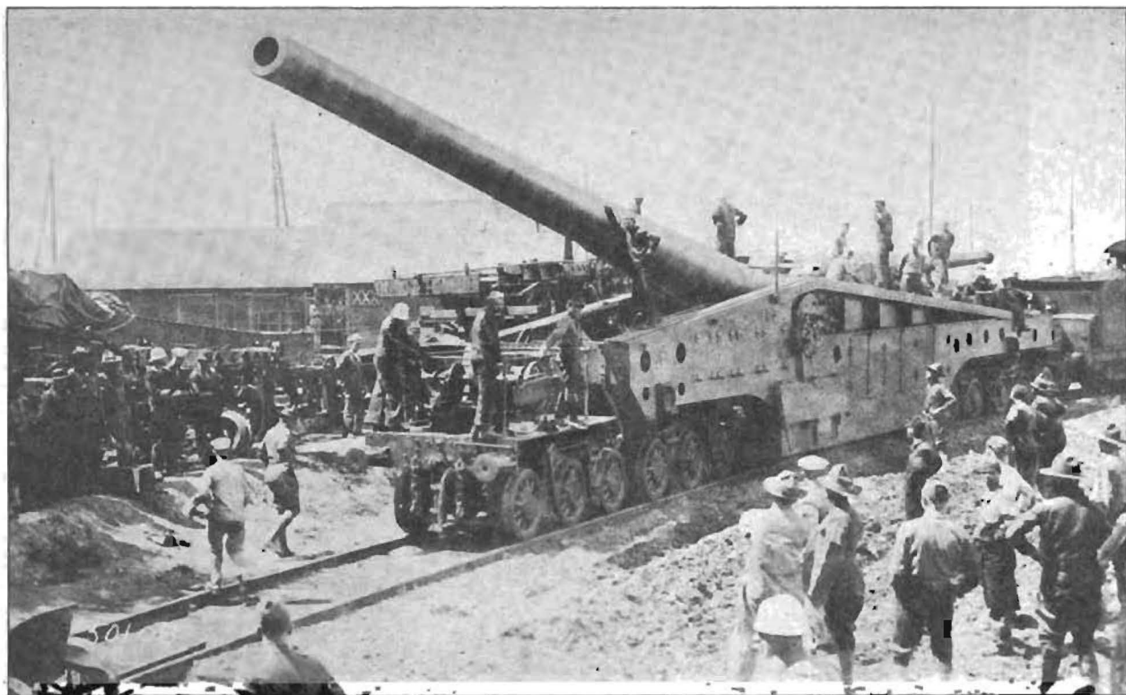
14-INCH, 50-CALIBER AMERICAN NAVY GUN MOUNT, MARK I, PARTIALLY ERECTED IN THE CHANTIERS DE LA LOIRE, ST. NAZAIRE, FRANCE.
