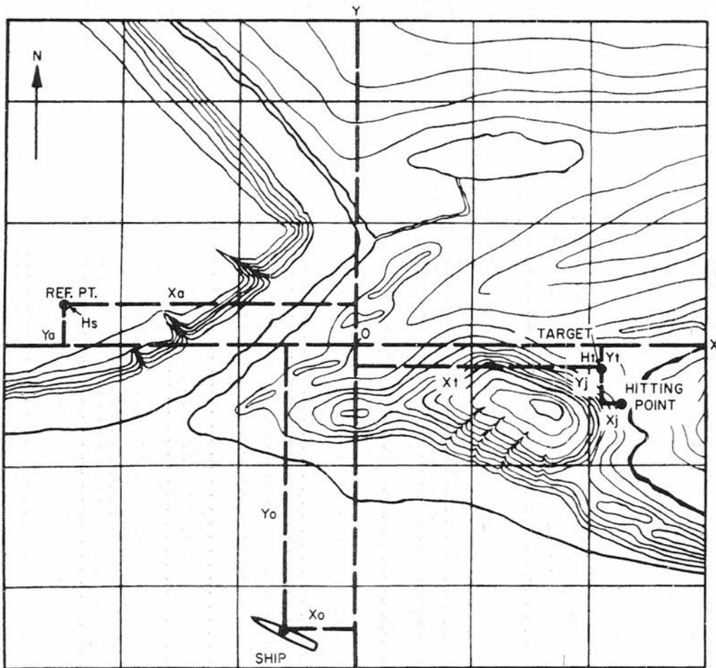
Figure 15. Horizontal Quantities Obtained from Plotter and Map
